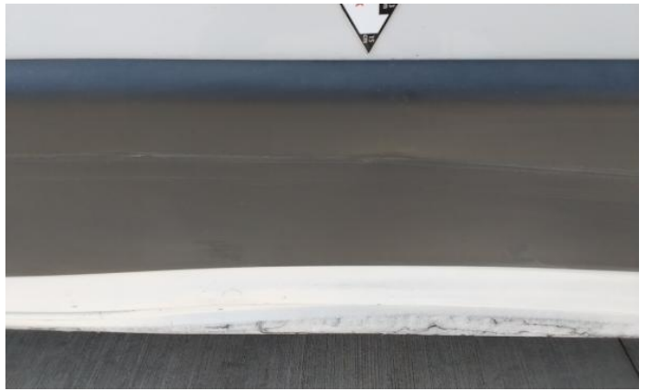
4: Qtr Panel nsr Chipped Edge Chip
